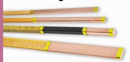
Special insulation materials, such as Glass yarn, Polyester-Glass yarn and Kapton, are lapped on bare conductors/tube or enameled wire for both rectangular and round wire and then, impregnated with epoxy.
